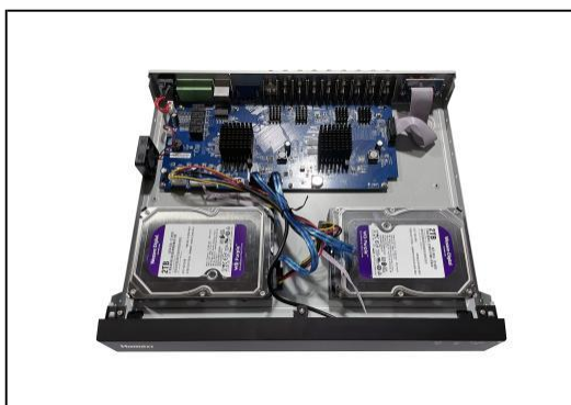
Figure 7 Connect the power and data cables
