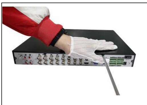
Figure 1-8 Install the cover and screws
